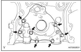
(c) Remove the 7 bolts, then remove the oil pump cover, drive rotor and driven rotor.
